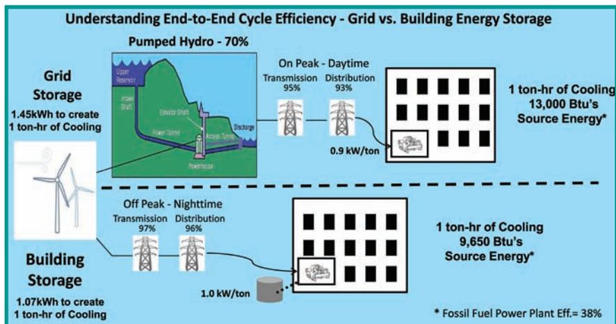
Figure 5: Energy storage and source energy for cooling.
